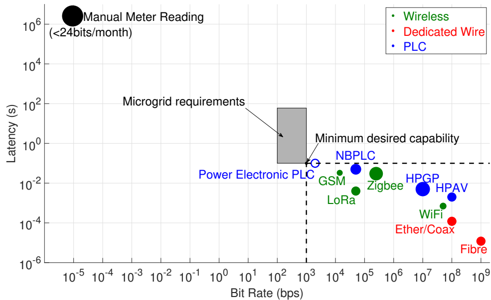
Figure 4.1: Microgrid FAN communication technology bit rate versus latency comparison. The filled dot area is scaled to reflect cost-per-customer (Power Electronics PLC is ‘free’ and so is an open dot). The grey rectangle shows the specification region that satisfies all three levels of hierarchical microgrid control. All the digital technologies from Table 4.1 exceed these requirements. The non-digital case of manual meter reading is included for comparison.
