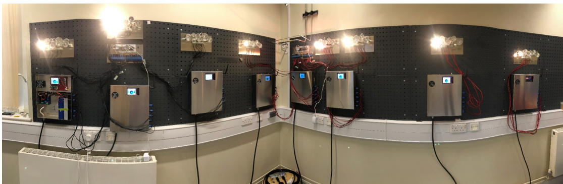
Figure 3.6: Laboratory microgrid testbed. Eight Homeboxes are connected to a central generation hub with various lengths and configurations of SWA cable.
