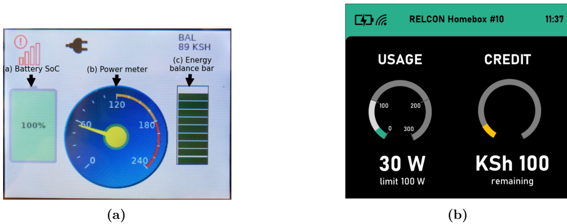
Figure 3.9: Two versions of the RELCON Homebox IHD which include a SOC indicator for the local lithium-ion battery, how much power the customer is currently using, PAYG energy balance, and connection status indicators for power and communication with the hub.
