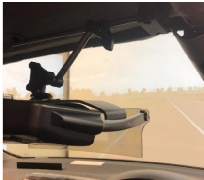
Figure 31. One of the Pioneer HUDs on an extendable arm within the driving simulator
