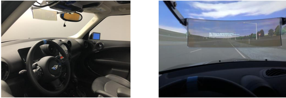
Figure 17. (Left) The Pioneer HUD within the driving simulator, and (Right) the HUD's appearance from the drivers' seat perspective (displaying text).
