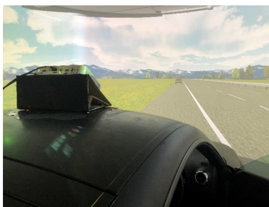
Figure 8. A projector positioned on top of the driving simulator cab to present a simulated HUD over the also projected driving environment.
