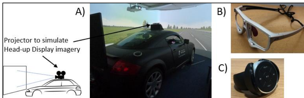
Figure 47. The materials used within the study. The driving simulator and projection-based simulated HUD (A) the SMI eye-tracking glasses (B) and the KWmobile Bluetooth button which was attached to the right side of the steering wheel (C).
