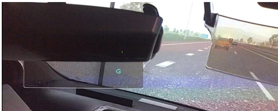
Figure 32. The letter "G" presented in position 4 on the second Pioneer HUD captured by the forward eye-tracking glasses camera. The body of the projection system obscures the driver's view of the slip lane.
