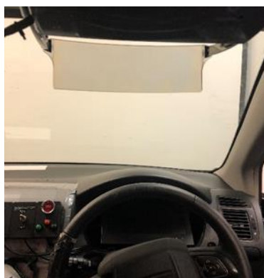
Figure 7. A Pioneer HUD attached to the ceiling of the vehicle cab. The combiner screen is visible as a clear rectangle near the top of the windshield. The projection system is positioned flat against the vehicle's roof.
