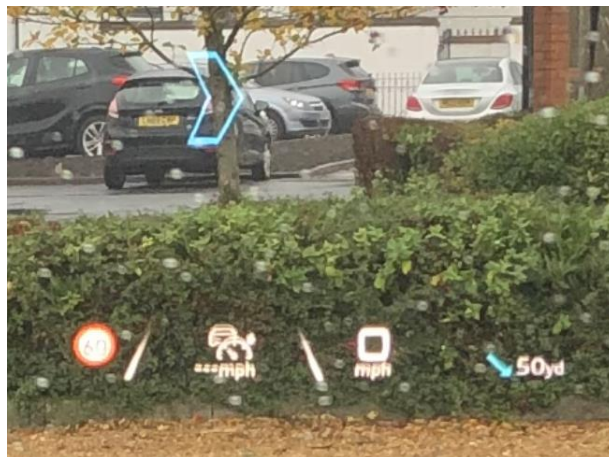
Figure 2. An example of a current HUD in and Audi Q4 E-Tron 2021. It contains speed information and navigation information, including a screen-fixed Augmented Reality (AR) arrow.
