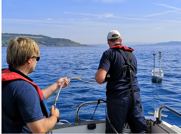
Fig. 1. A step of the deployment of the digital thin line array behind the AutoNaut USV. After attaching to the stern of the vessel, two operators gradually feed the array into the water from a support vessel.
