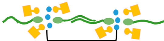
Figure 5. A schematic depicting the proposed DES structure with the CSA shown as yellow blocks, the sulfobetaine shown in green, and the water as blue circles. The black bracket depicts the repeating unit that gives rise to the d -spacing.
