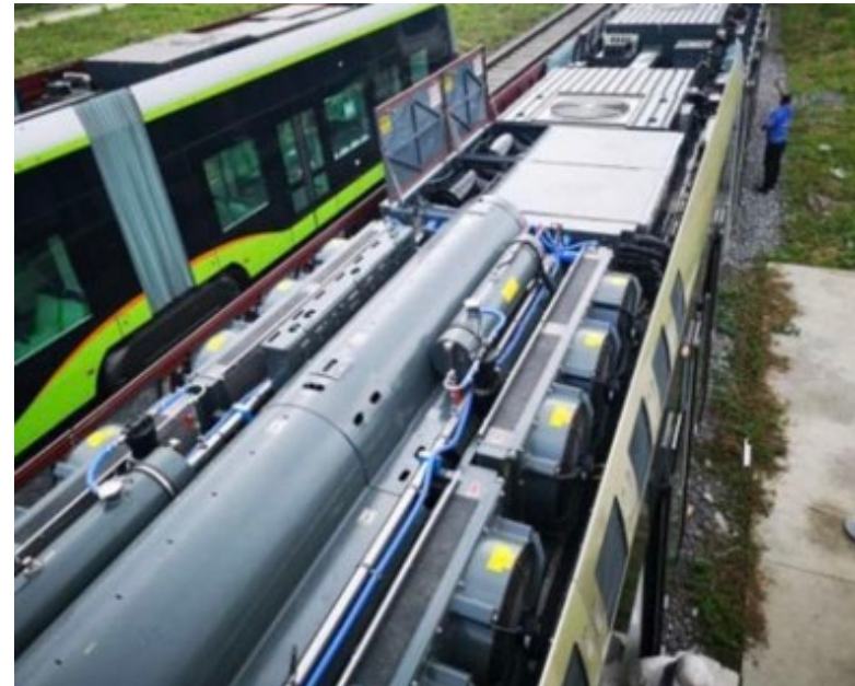
Hydrogen tank and Ballard fuel cell system on CRRC-Sifang light rail - https://blog.ballard.com/fuel-cell-trains
