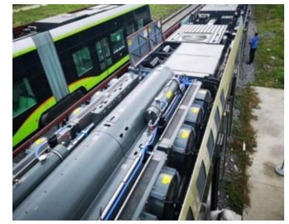
Hydrogen tank and Ballard fuel cell system on CRRC-Sifang light rail - <u>https://blog.ballard.com/fuel-cell-trains</u>
