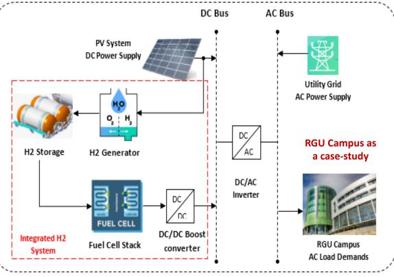
Proposed Zero-Carbon Hydrogen-based Grid-connected Building Scenario
