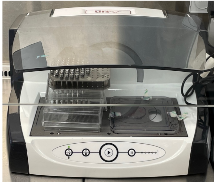
Figure 2.1: Mast URI dot machine, with the 96-multipin inoculator head fixed in place with 52 pins inserted. This image details the stage at which the MPI head was being sterilised in 90% ethanol prior to use
