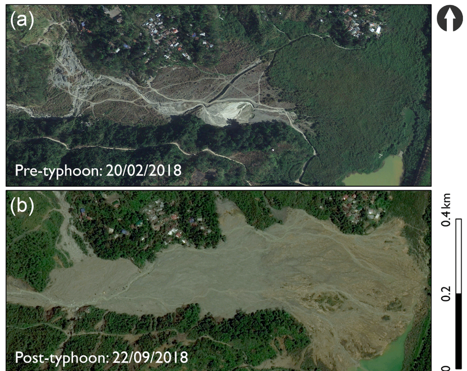
FIGURE 3 - Sedimentation of TSF2 between 20/02/2018 (a) and 22/09/2018 (b). Image Centre is 16.39750°N 120.67473°E. Source: Google Earth.
