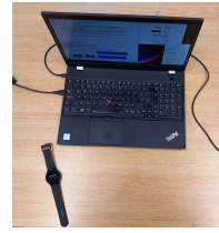
(a) RadioMe Prototype System Setup: the system runs on a laptop to which a smartwatch sends heart rate and motion sensor data.
