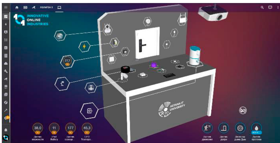
Fig. 3. Digital twin of the “Smart Home” testbed and Home Assistant platform control panel
