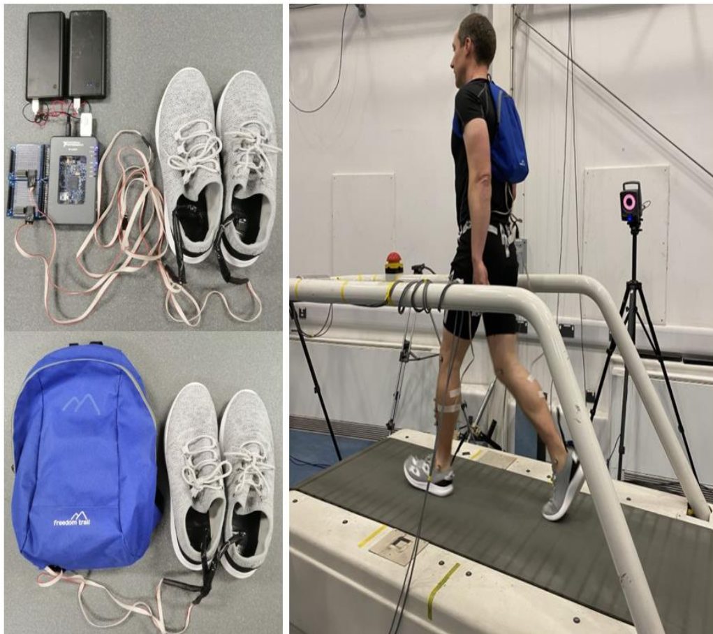
Figure 9 Temperature assessment set up while walking on the treadmill
