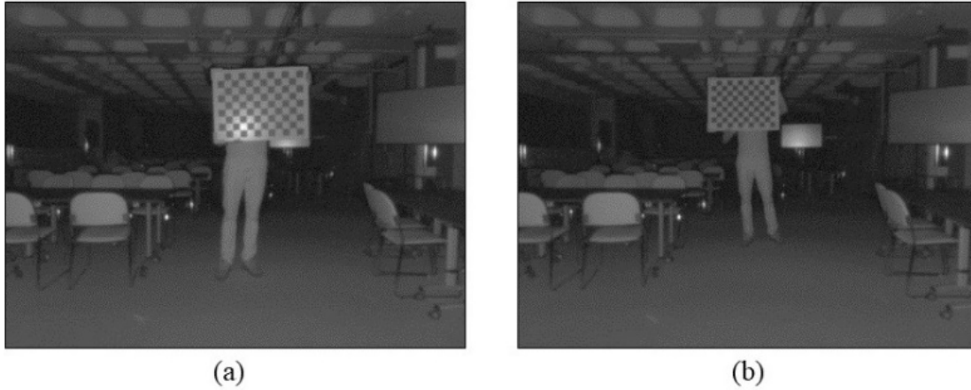
Fig. 82: (a) Glare from flash lidar intensity data which can degrade calibration and (b) use of various target angles to capture images without glare. Reproduced from [4].
