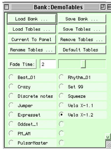
FIGURE 2.6: The TABLE BANK window allows storage, recall and editing of sets of table data. The window also provides control over user-defined interpolation between data sets
