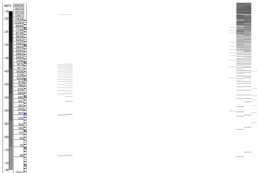
FIGURE 2.3: A spectrogram in dBV (logarithmic frequencies, analysis window size = 2048) of a pulsar to pulsarLET conversion. Notice not only changes in the frequency domain but also widened temporal region - here visible as an increase from 2 to 4 columns
