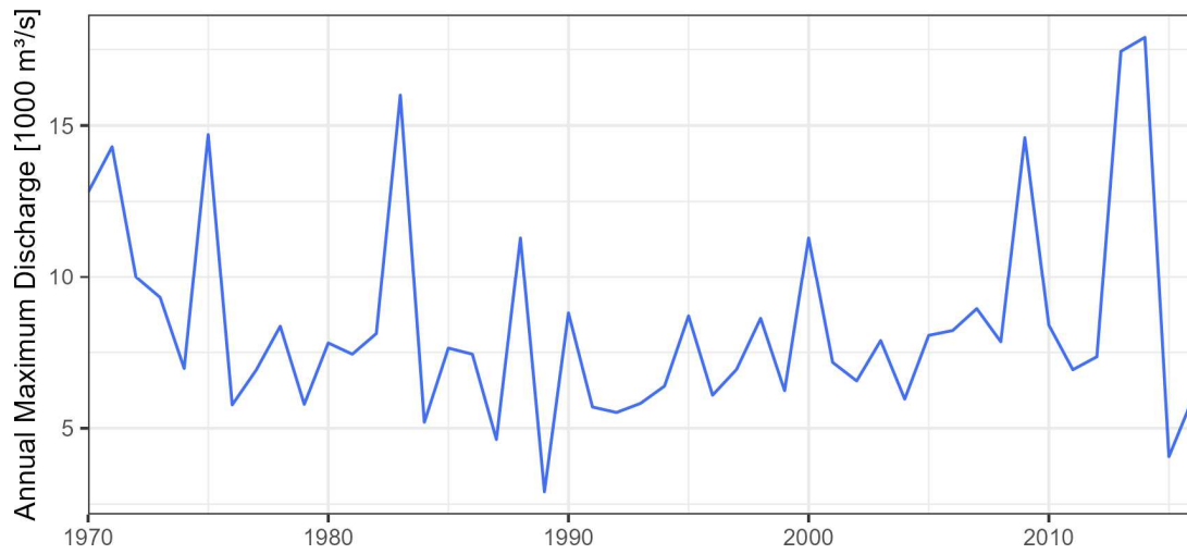
Figure 2.7: Annual Maximum Flows recorded at the mountain outlet. The gauging station is maintained by the Department of Hydrology and Meteorology, Nepal.
