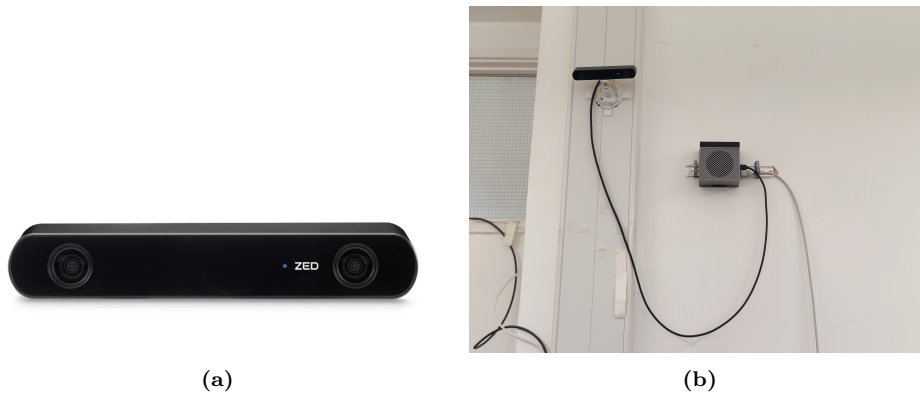
Figure A.6: ZED 2 camera from Stereolabs (a) and its location on the wall (b)
