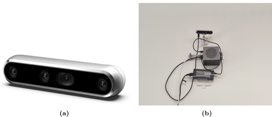
Figure A.7: Intel RealSense Depth Camera D455 (a) and its location on the wall (b)
