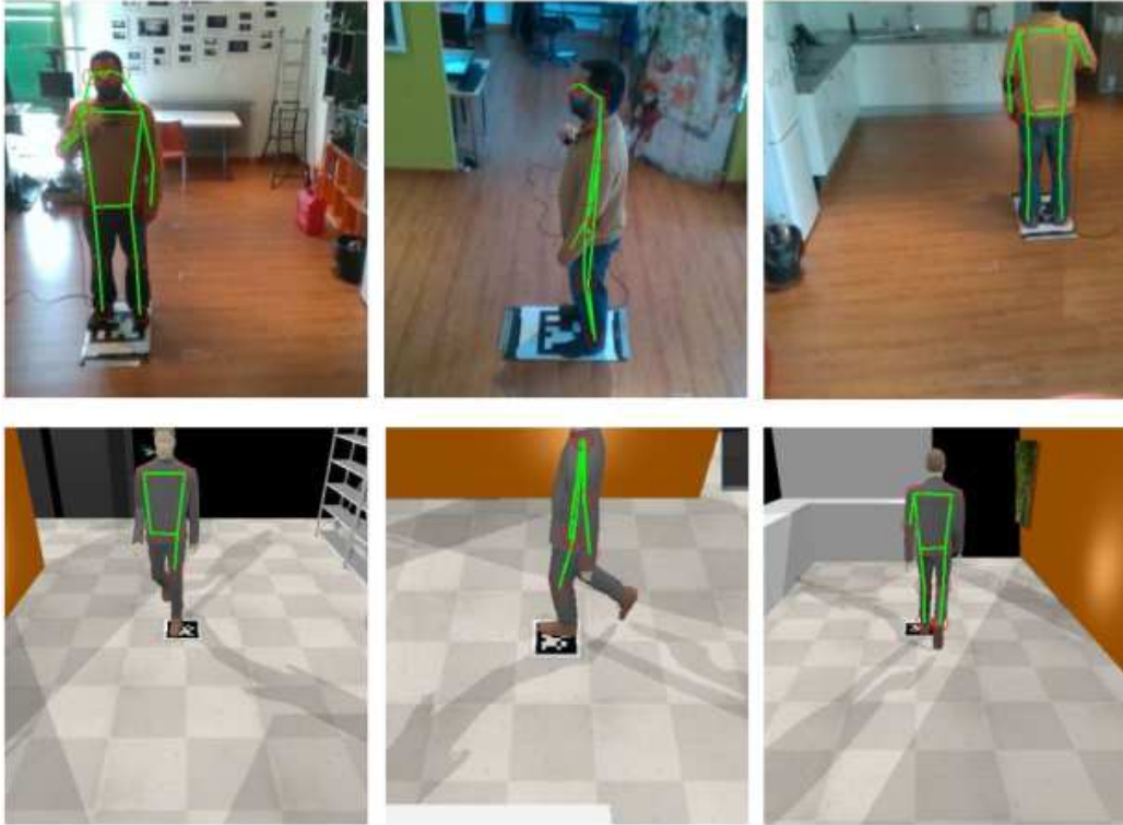
Figure 6.1: Example of real images (first row) and images obtained from the simulator (second row). The resolution employed in the experiments was 640x480. Skeleton detection is visualized with green lines, highlighting the keypoints and connections between them for both real and simulated images.
