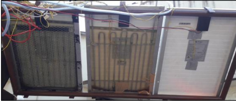
Figure 2-8 PV Model of PCM with and without aluminium matrix with reference PV adapted from [86].
