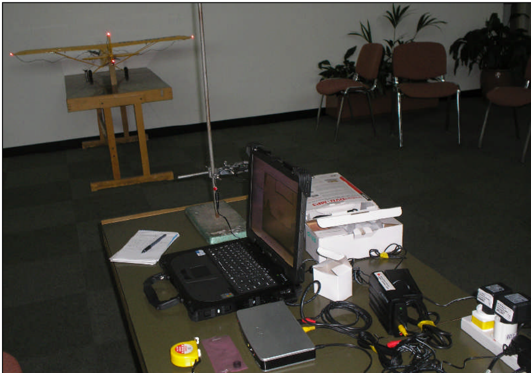
Diagram E3.1: Indoor experiment set up, showing camera aligned with model aircraft
