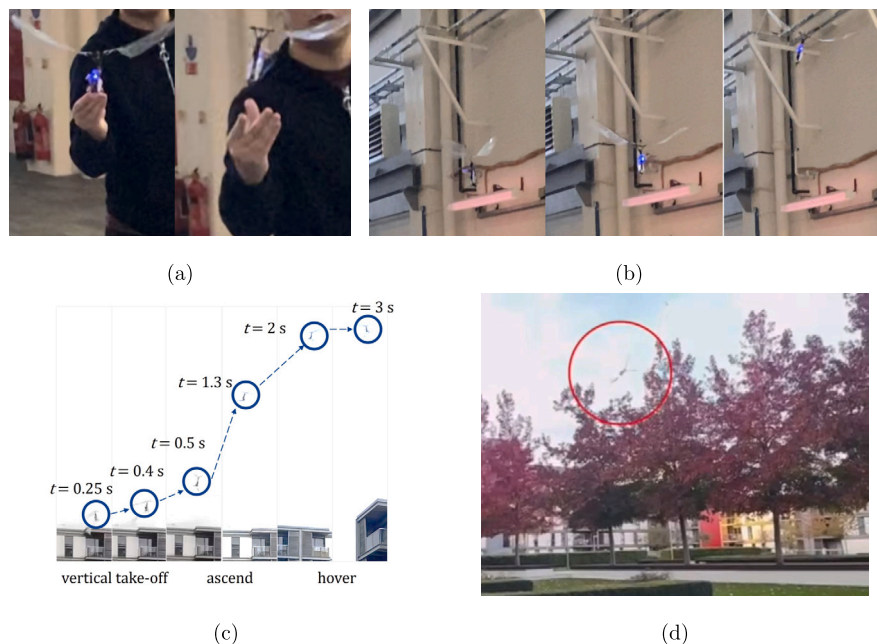
Fig. 22. Single-motor FWR-MAV model with dragonfly-like wings: (a) free launch from hand; (b) vertical take-off in indoor test; (c) outdoor test; (d) Dual-motor FWR-MAV model outdoor test.
