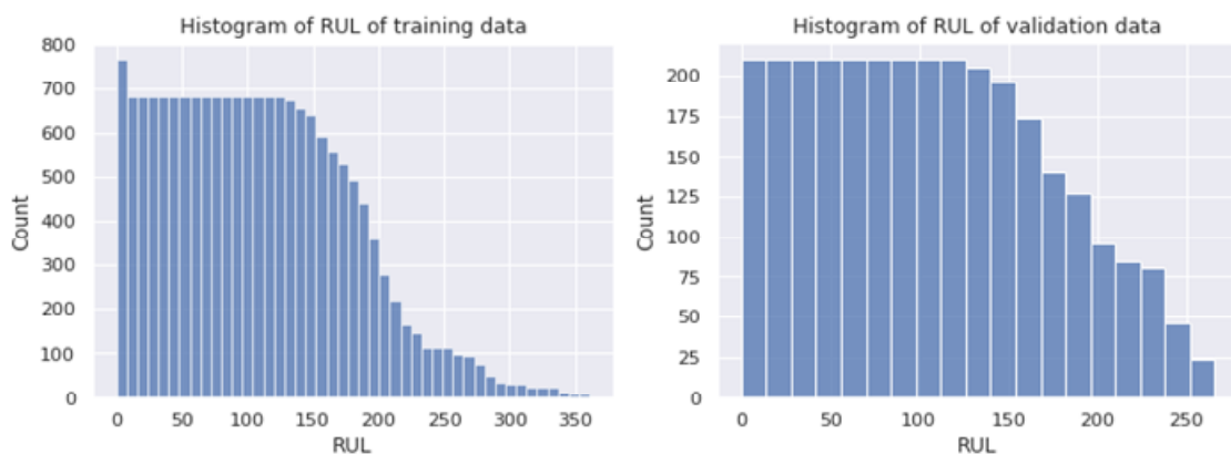
Figure B-4 Plot comparing the distribution of RUL values for the units in the training data to those in the validation data.
