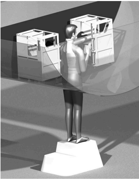
Figure 6: Redesigned A-8 Avionics Bay with 5 th Percentile Maintainer.
