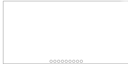
Figure 2. Cross-section of the computational domain with a lateral array of 9 actuator discs. The height and width of the domain are 25d and 50d , respectively, the lateral gap between each disc is 0.5d , and the vertical gap between the discs and the ground is also 0.5d .
