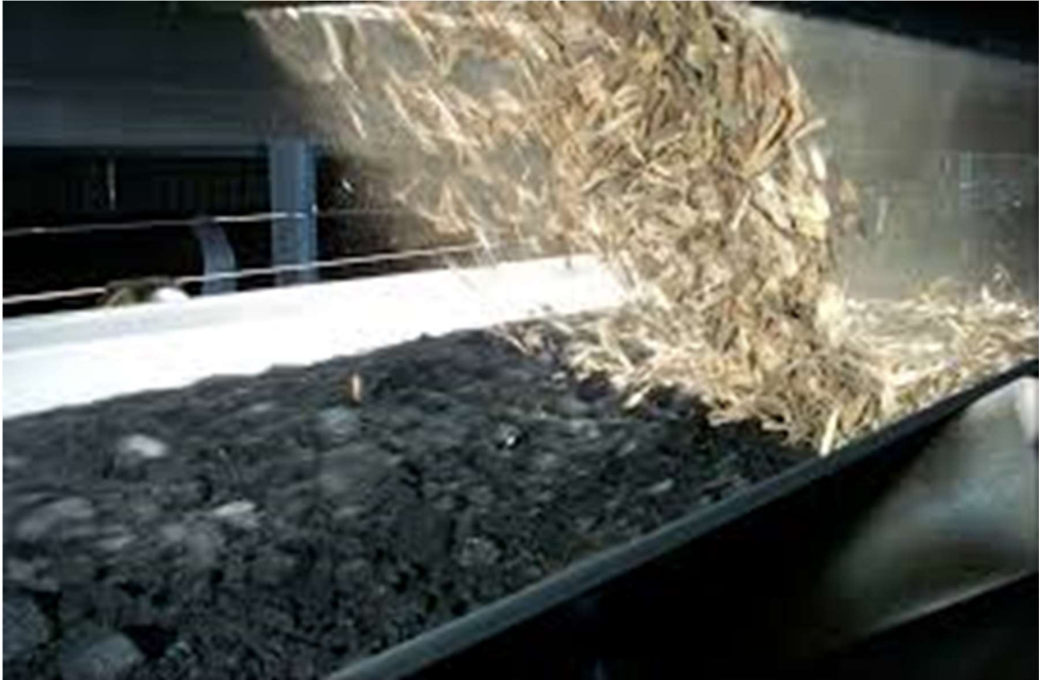
Figure 2-10 Direct addition of woodchips on a coal conveyor at Wallerawang Power Station, Australia (Koppejan and Baxter, 2013)
