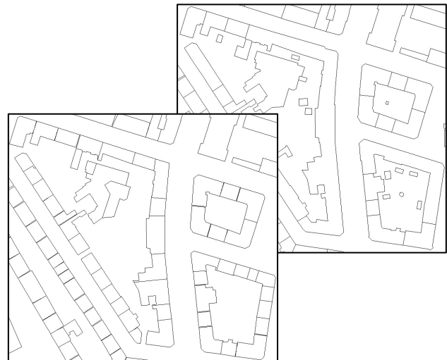
Figure 10. The background upper picture shows a snapshot of raw footprints from the technical map. The lower front picture shows the resulting shapes of these footprints when cut by polygons of cadastres.
