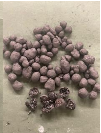
Fig. 7.6. Procedure PCM impregnated LWAs preparation
