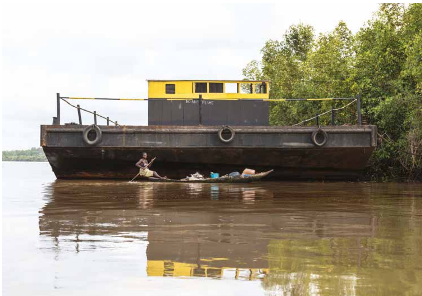
Barge (stationary) used for loading crude oil and refined automotive gas oil (AGO) in a tight creek area.
