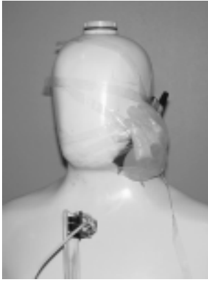
Figure 2: One of the handsets mounted for measurements with the HHP.
