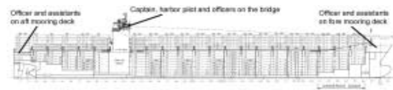
Figure 4: Distribution of co-workers on Sally Maersk during the operation of letting go the lines.
