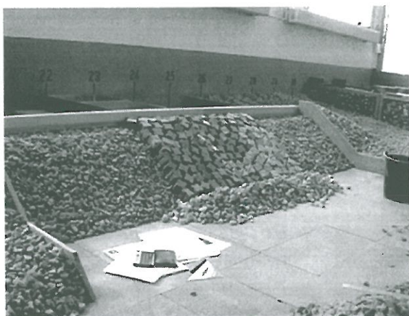
A) Breakwater model during construction.
