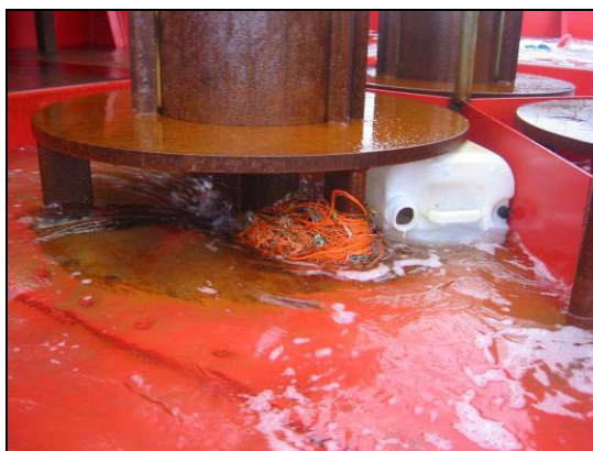
Fig. 4.3 Debris collecting at the dummy turbine cylinder gate
