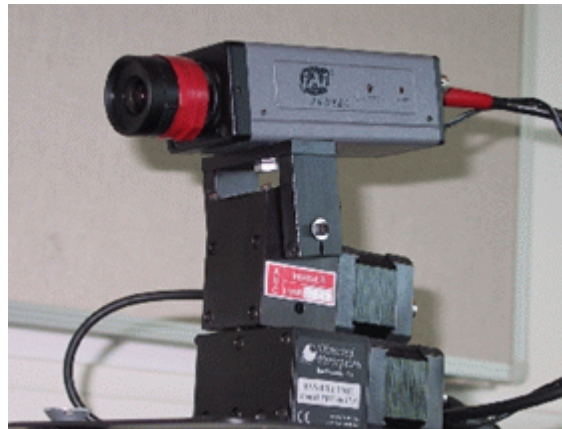
Figure 3.6: The figure represents an example of monocular camera head (the one used for the experimentations presented in next chapters).
