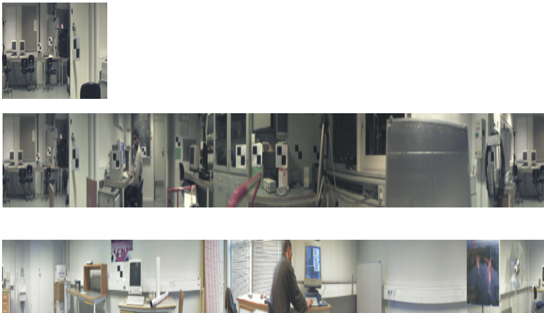
Figure 5.4: The figure top-row shows a computed panoramic view which has been synthesized by projecting 10 images of 350x350 pixels each, over 60 degrees, (i.e. 1 image every 10 degrees rotation). The figure middle-row shows a panoramic view of the same workspace but synthesized projecting 72 images of 350x350 pixels each, over 360 degrees, (i.e. 1 image every 5 degrees rotation). The overlapping area between two adjacent images is in this case about 85%. Maximum overlap is 7 images contributing to the same pixel in the panorama. The figure bottom-row shows a panoramic view of a different workspace, which is still synthesized by projecting 72 images over 360 degrees, but the size of each image is 256x256 pixels. The entire image was 256x4101 pixels.
