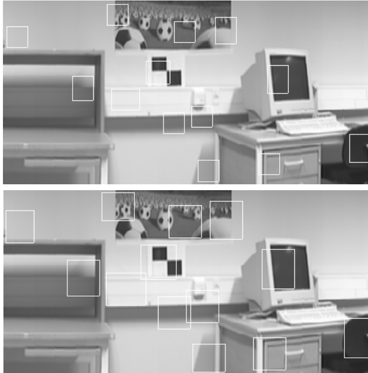
Figure 5.18: The figures show results of experiments aimed to confirm the proposed ideal size by testing extraction of landmarks having different texture-template size. In particular the figure bottom-row shows the case when the template size is increased up to twice the ideal template area. Extracted landmarks were for most of the cases the same as extracted with the ideal size setup, which confirmed reliability of the ideal size.
