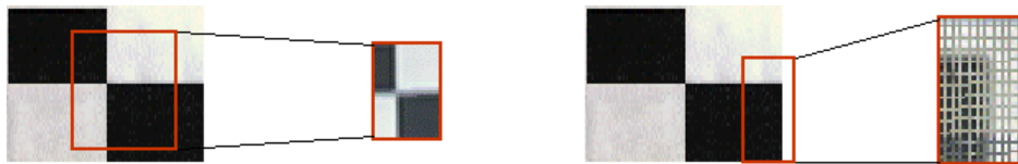
Figure 4.6: The figure shows example of computed landmark visual predictions, both in case of compression and enlargement, emphasizing undesired mapping problems.
