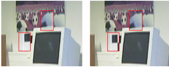
Figure 6.15: The figure shows examples of generated visual predictions superimposed to current observations. The left-hand side shows two visual predictions reconstructed based on one representative reference-view only, (previous method). The right-hand side shows visual predictions reconstructed by two reference-views, (proposed method). The reconstructed views in the right-hand side show a slightly larger wall portion.
