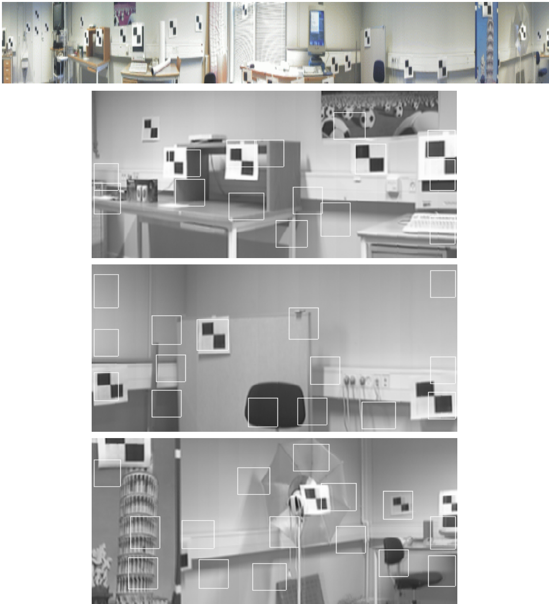
Figure 5.17: The figures show results of experiments aimed to test extraction of landmarks having different orientations. To this purpose the workspace was filled in with plenty of "ideal" texture patterns. The figure top-row shows the experimental setup through a panoramic view. The figures in the three rows from the bottom shows typical extracted landmarks. The ideal landmark is always selected when its dimension in the image-plane approximately occupy over 70% of the template ideal size. If the projected region is larger then the ideal size a part of "ideal" landmark is always selected.
