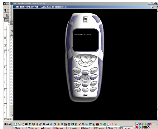
FIGURE 20. The simulated “Fakephone” Webbased GUI used to display the textual output. The phone “display” will automatically update e.g. once per second and runs in any web browser.
