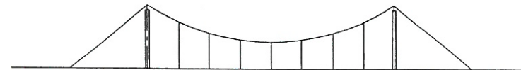
(f) Staying with transverse cables to ground or to another part of the structure
