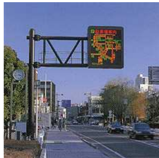
Figure 5: Japanese parking guidance graphical information sign (source: Nagoya Electric Works Co. Ltd.)
