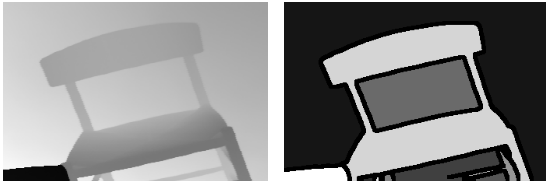
Figure 3. A Range image (left) and corresponding extracted regions after labelling.
