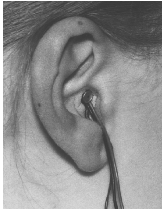
Fig. 4. Example of a microphone technique for blocked-entrance binaural recordings. A hole of suitable size is made in an EAR earplug – for instance by a soldering iron – and a Sennheiser KE 4-211-2 miniature microphone is inserted in the hole. The earplug, with the microphone inside, is then compressed and, once well compressed, earplug and microphone are inserted into the ear canal. Earplug and microphone should be held in position while the earplug decompresses, so that the microphone is ensured the correct position flush with the entrance – after [76]
