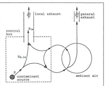
FIGURE 2. Control box to distinguish between directly captured and escaped contaminants. The circle to the right represents room air excluding the control box.
