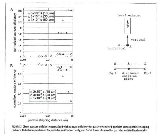
local exhaust cannot be described by particle stopping distance alone.
