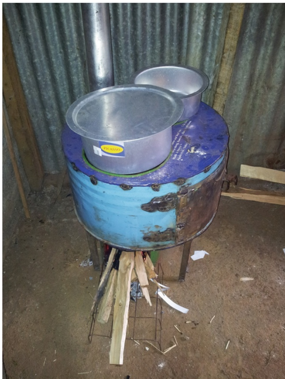
Figure 5 Locally constructed, improved cookstove installed in Kenya.
