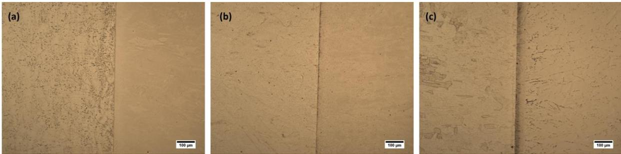
Figure 17: Etched optical micrographs of the interface microstructure of SS316L vs IN718 diffusion couples annealed at (a) 850 °C for 120h, (b) 950 °C for 48h, and (c) 1050 °C for 24h followed by WQ.
