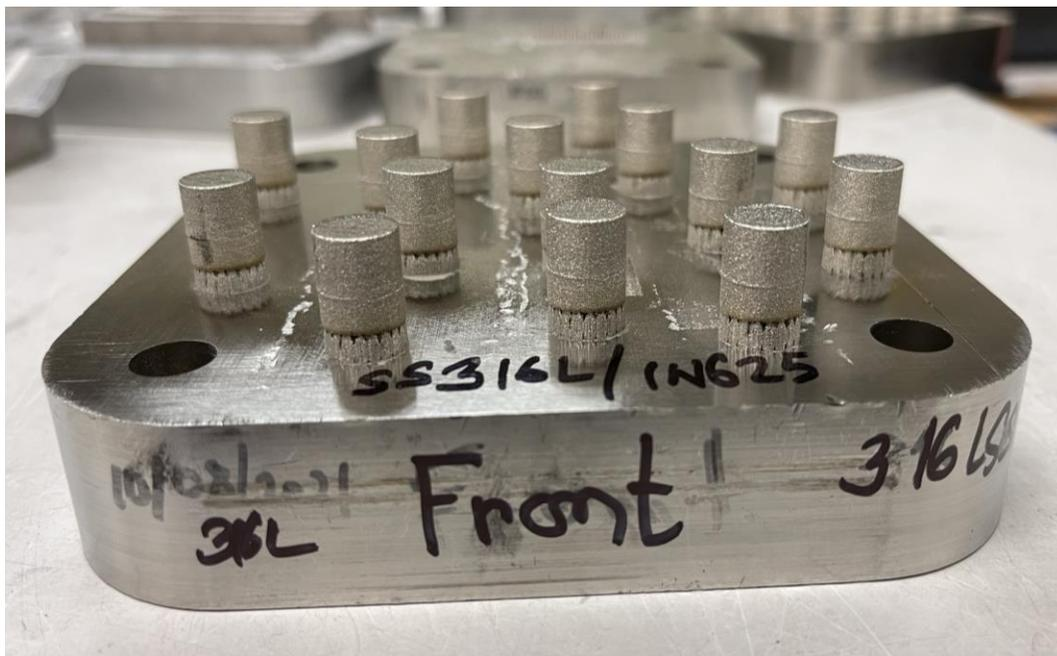
Figure 4: Fabricated SS316L/IN625 bimetallic structures. The diameter and height of the cylinders were 10 mm and 12 mm, respectively.
