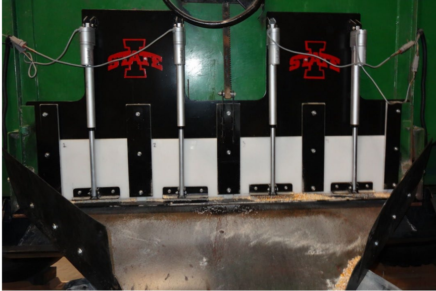
Figure 3: Yield system test stand metering gate with positional feedback gate control
