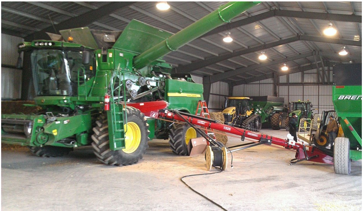
Figure 2: Yield system test stand feeding grain into harvester clean grain system
