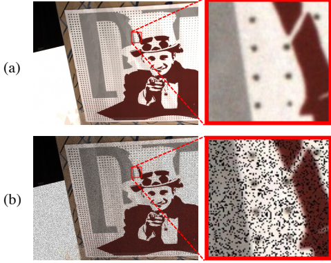
Figure 4. Image-level contrastive sample. (a) a source image of the regular sample. (b) a source image of the image-level contrastive sample. A Bernoulli-distributed binary mask is used to simulate the failure case of local photometric consistency in (b).
