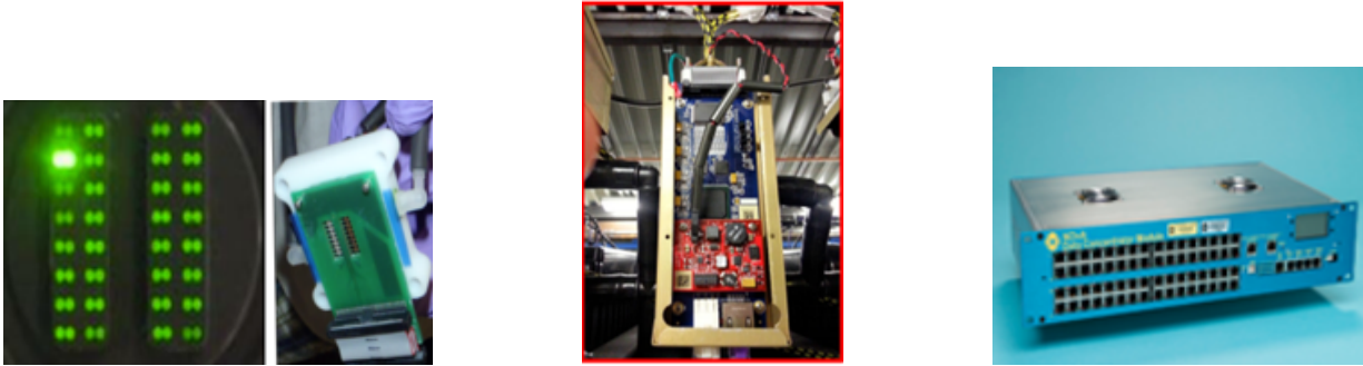
Figure 2.7: A picture of APD (left) where the ends of 32 wavelength-shifting fibers are collected at the end of scintillation cells, FEB (middle) and DCM (right).
