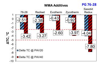
ΔTc Values at PAV20 and PAV40 Oxidation Levels: (a) PG 76-28, (b) PG 58-28
