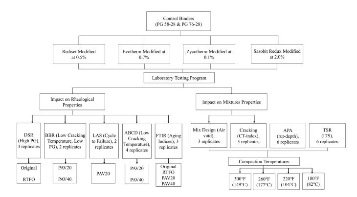
*Note.* DSR: Dynamic Shear Rheometer; BBR: Bending Beam Rheometer; LAS: Linear Amplitude Sweep test; ABCD: Asphalt binder Cracking Device; FTIR: Fourier Transform Infrared Spectroscopy; CT-index: Crack tolerance index. RTFO = rolling thin film oven; PAV = pressure aging vessel
