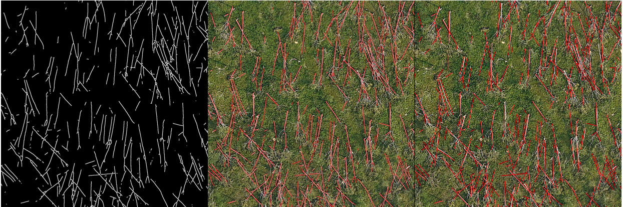
FIG. 13. (left) Preprocessed treefall segmentation mask, (center) extracted edge lines using fast line segment detector (van Goi et al. 2010), and (right) joined lines using the constructed line-joining algorithm, for the 64 m × 64 m section of the Alonsa, Manitoba, tornado shown in Fig. 10.
