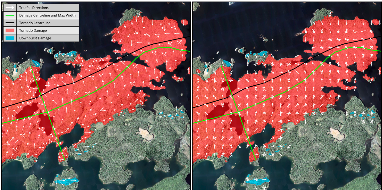
FIG. A1. (left) Manual and (right) automated TrIDA maps for a 4.25 \text{ km} \times 4.25 \text{ km} section of the Brooks Lake, Ontario, tornado with a 250-m grid size. This section of the Brooks Lake tornado does not overlap with any images used for training or validation of the automated model.
