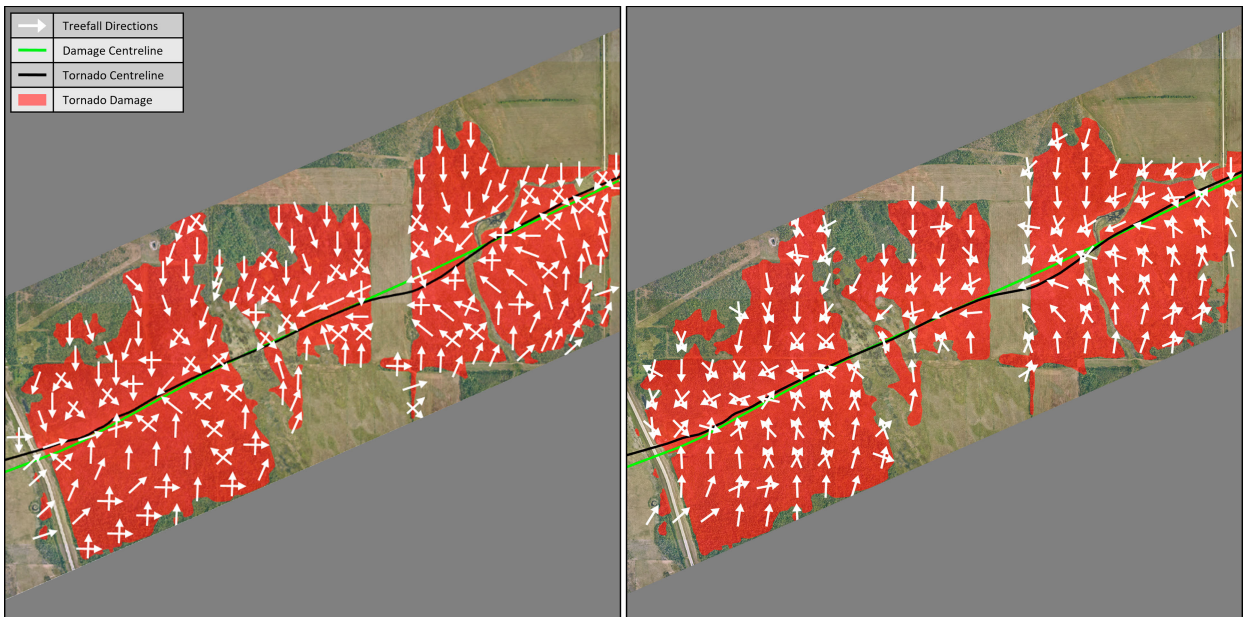
FIG. A2. (left) Manual and (right) automated TrIDA maps for a 2.6 \text{ km} \times 2.6 \text{ km} section of the Alonsa, Manitoba, tornado with a 120-m grid size.
