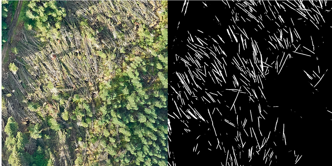
FIG. 11. (left) A 64\text{ m} \times 64\text{ m} image of the Lac Gus, Quebec, tornado and (right) automatically extracted mask.
