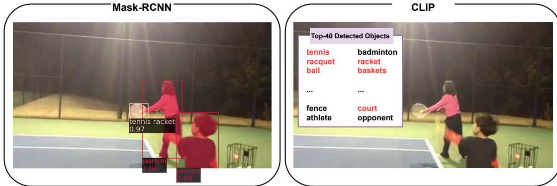
Figure 2.2: A comparison between objects identified using Mask-RCNN (He, Gkioxari, et al., 2017) (on the left) and CLIP (on the right) is illustrated in the following images. Our Attention Mechanism Module (AMM) highlights the most pertinent objects, which are emphasized in bold red .
