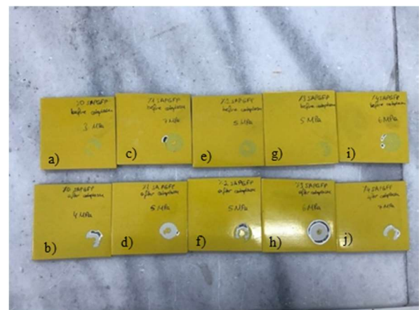
Fig.7. Pull off test results for (a) 0% SAPGFP-before aging, (b) 0% SAPGFP-after aging, (c) 1% SAPGFP-before aging, (d) 1% SAPGFP-after aging, (e) 2% SAPGFP-before aging, (f) 2% SAPGFP-after aging, (g) 3% SAPGFP-before aging, (h) 3% SAPGFP-after aging, (i) 4% SAPGFP-before aging, (j) 4% SAPGFP-after aging
