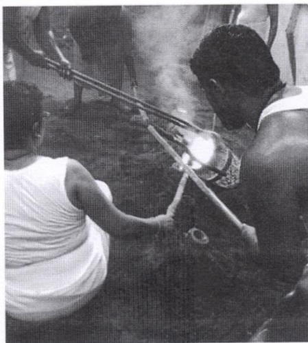
Fig. 6. Metal icon casting at Swamimalai, Thanjavur district, Tamil Nadu
