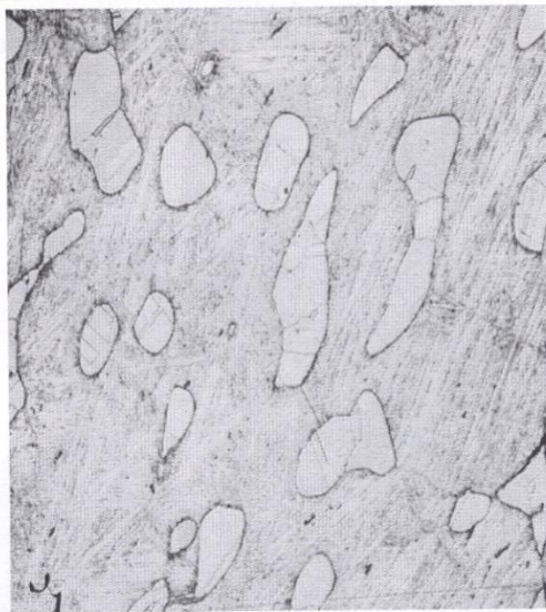
Fig. 8. Micro-structure of vessel from Adichanallur, Government Museum, Chennai, hot forged/wrought and quenched high-tin beta bronze structure of 23.9 % tin bronze, 400 X
