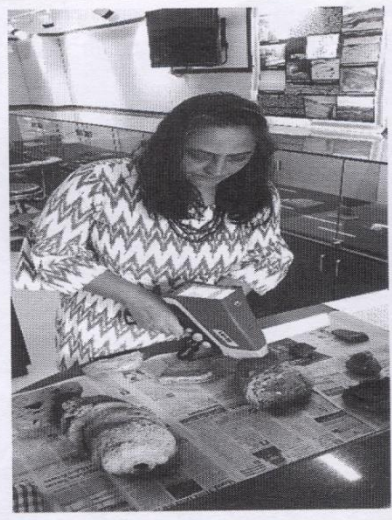
Fig. 14. Exploring zinc smelting retorts using portable XRF analysis at NIAS Lab procured under Prof. Sharada Srinivasan's DST-SHRI project
