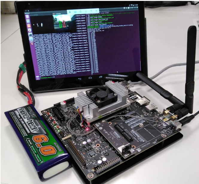
Fig. 1. Embedded solution: Jetson TX2 development kit is battery powered and remotely controlled using a tablet and WiFi connection.
