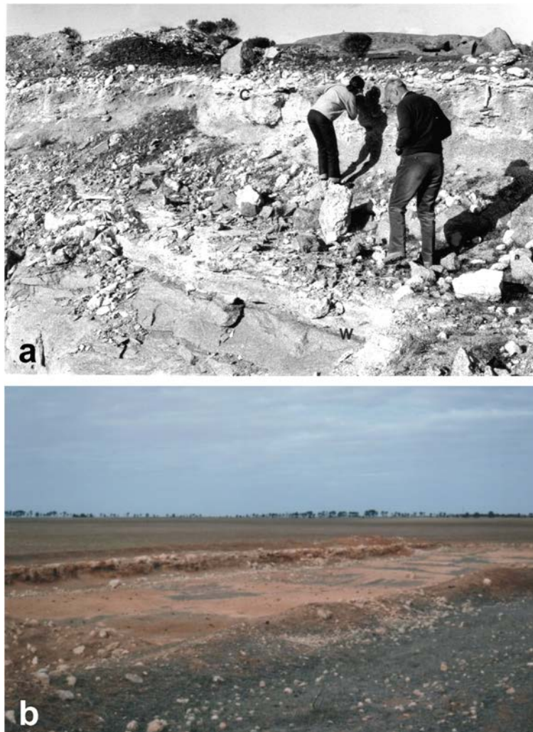
Figure 3. (a) Quarry section of regolith on granite, but with substantial protective capping of calcrete derived from airborne carbonate dust. (Explanatory notes. (S. M. Kraemers, pers. comm. 1983) Surface 0-10cm red sandy soil; 10-20 cm nodular calcrete with granite fragments and quartz grains; 20- 24 cm massive calcrete; 24-30 cm nodular calcrete; 30-60 cm grus and clay, lenses of calcrete; 60-90 cm laminated grus and clay; 90-91 cm bleached rock; 91-92 cm fresh granite; 92-93 cm iron -enriched granite; 93cm- fresh granite) (b) massive duricrust.
