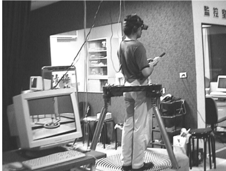
Figure 24: Omnidirectional ball-bearing disc locomotion device. Source: Huang (2003).
