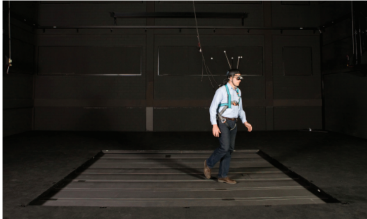
Figure 23: CyberWalk, an improved Omni-directional treadmill. Source: Souman et al. (2011).
