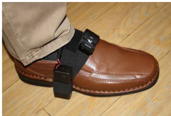
Figure 36: Sensor attached to the shoe using tailor-made straps. Source: de la Rubia and Diaz-Estrella (2015).
