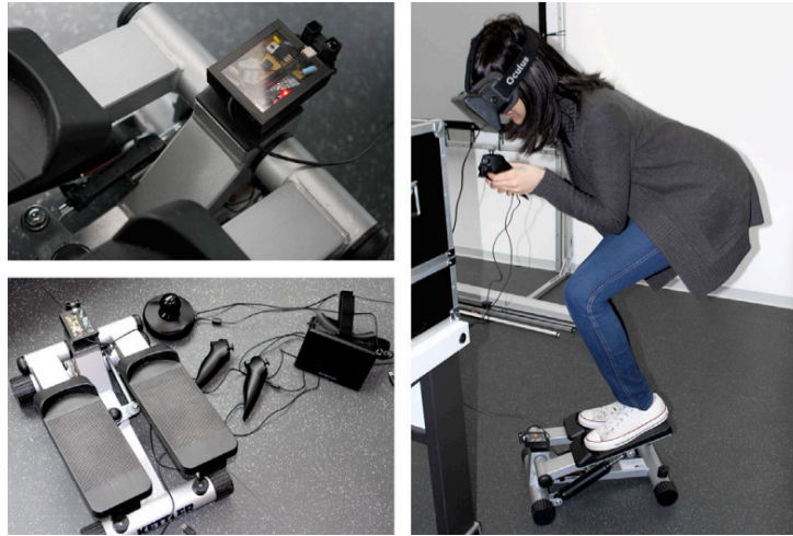
Figure 30: User crouching while using a VR-Stepper for locomotion. Source: Matthies et al. (2014).
