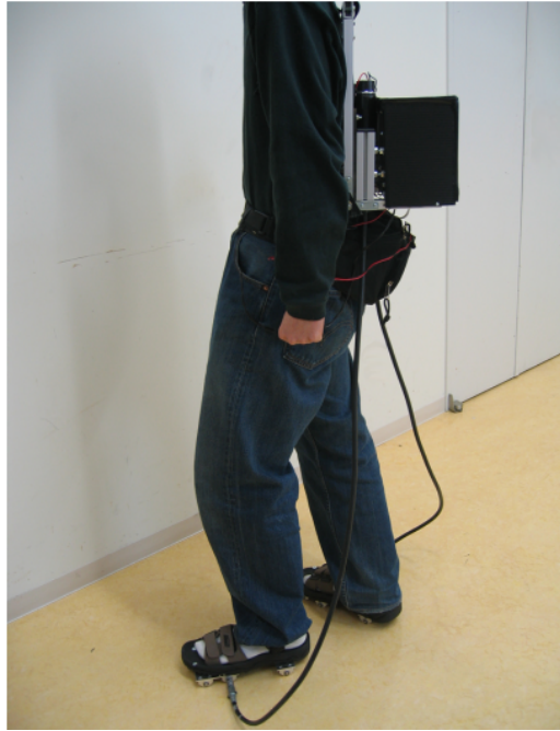
Figure 37: Overall view of the Powered Shoes. Source: Iwata et al. (2006).
