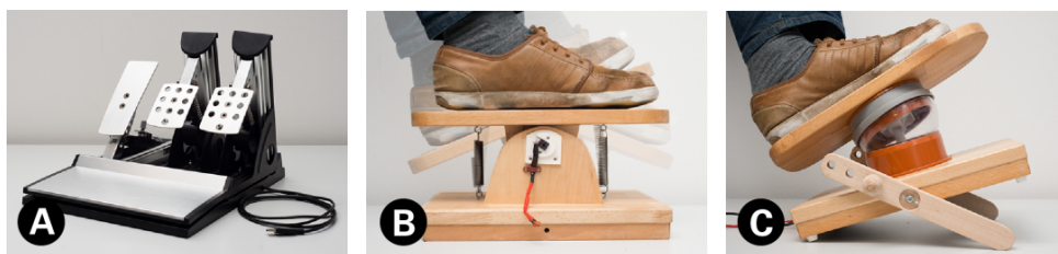
Figure 34: a) One-directional Pedals, b) Two-directional FootRocker and c) Multi-directional Foot-Joystick. Source: Klamka et al. (2015).
