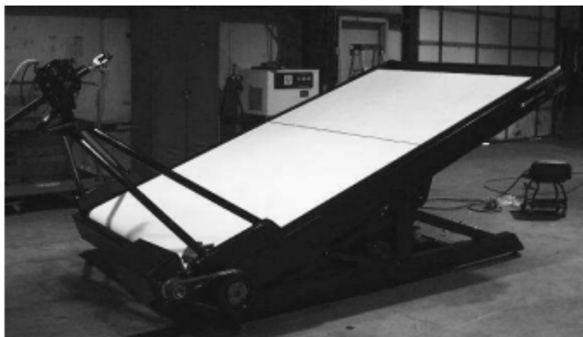
Figure 26: Tiltable treadmill at max capacity. Source: Hollerbach et al. (2000).
