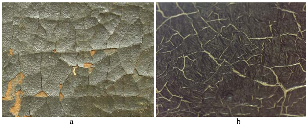
Fig. 3. Networks of craquelures: a - craquelures of age, in the sleeve over the chair; b - premature craquelures, in the green cloth, at the bottom.
